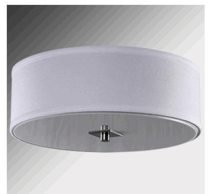
12" Brushed Nickel Ceiling Fixture, Two GU24 sockets, Direct Wire, with White Linen Hardback Shade with self fold trim and White acrylic bottom diffuser. Recommend two 800 lumen LED bulbs with GU24 base. 12" Diameter x 4"H
